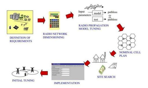
Figure 3. Radio Network Design Process
